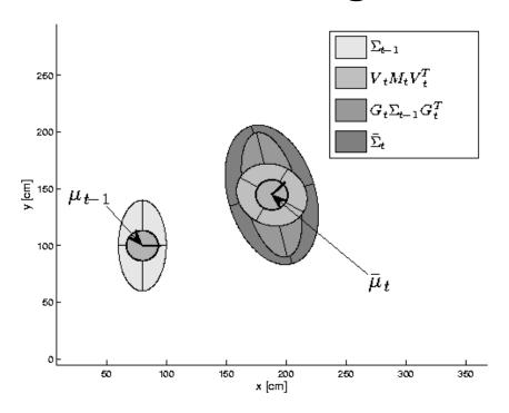
recall that in the prediction step the state mean and covariance are projected forward in time using the plant model
