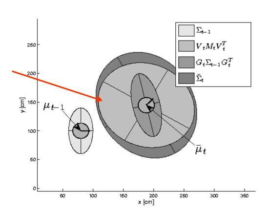
in the first part of the correction step, the measurement model is used to predict the measurement and its covariance using the predicted state and its covariance
